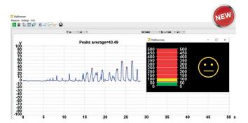
Body voltage measurement test set-up. The software "Digilloscope" can mark the five highest peaks automatically and calculates the average value.
