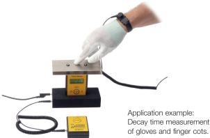
For resistance to ground measurement of gloves and fingercots.
