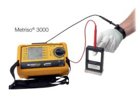
Application example: Resistance to ground measurement of gloves and finger cots.
