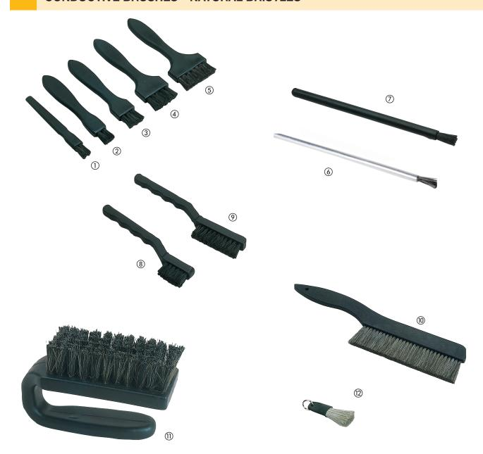
Our range of conductive brushes allows thorough cleaning of ESD sensitive assemblies without the danger of high charges generated by conventional brushes. They consist of a conductive plastic handle and bristles made of highly conductive fibers which will dissipate any charges by corona discharge, due to their small diameter. Natural hair is mixed with the conductive fibers to provide the desired stiffness. Includes the ESD Symbol.
