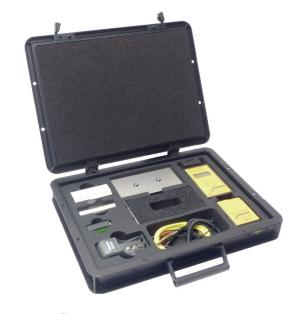
Verification Kit for measuring electrostatic fields and electrostatic charges, as well as the body voltage of a person while performing the walking test. Additionally the decay time and the offset voltage of ionizers can be measured.
