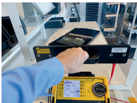
application example: measurement acrylic cover
