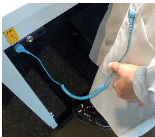
grounding via coilcord
